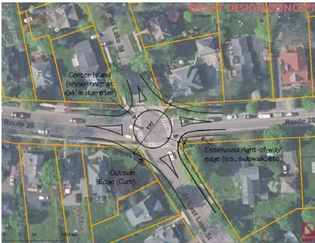
Figure 4.18: Draft design concepts for roundabouts at the U.S. 20 intersections with State Route 41A (top) and State Route 41 (bottom).
