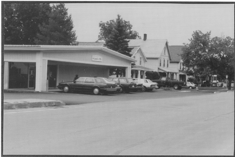
Discouraged: When street and parking lot are continuous, pedestrians lose their space.
